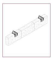
Gable restraint brackets placed on wall at 1200mm\* maximum centres (no fixings required).
