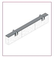
10mm maximum mortar bed on wall prior to wallplate being fixed.
